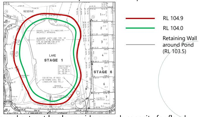
The tested cut-in and cut-out levels provide enough capacity for flood storage while maintaining an aesthetically acceptable pond level
