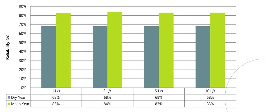
• The 2 L/s offtake is most applicable as it is the minimum offtake rate needed to irrigate Tally Ho Reserve in one irrigation cycle
