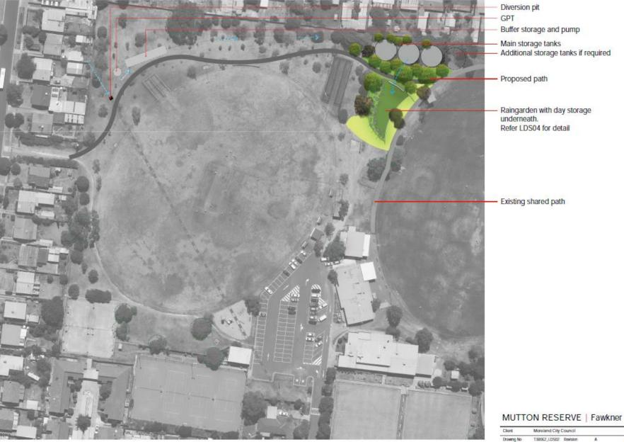
Buffer storage and pump - Main storage tanks - Additional storage tanks if required
